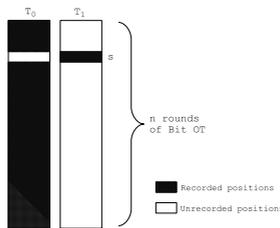
**Fig. 1.** During the  $n$  Bit OT executions Bob chooses  $t_c^i$  at positions  $i \in I \setminus s$ , and  $t_{\bar{c}}^i$  at positions  $i \in s$ . In the Figure,  $c = 0$  so in the end Bob knows  $T_0(I \setminus s)$  and  $T_1(s)$ . Note that while  $s \subset I$  is shown here as a contiguous block, in reality the positions it represents occur throughout the  $n$  executions.
