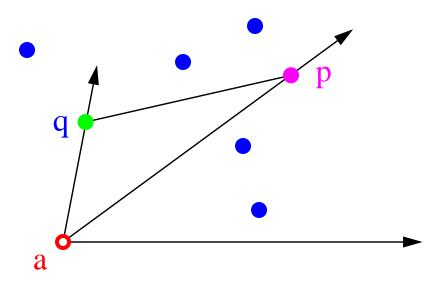
$\theta(p) < \theta(q) \iff \text{orientation of } (a,p,q) \text{ is counterclockwise}$
