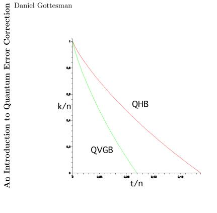
THEOREM 4. A quantum [[n, k, d]] code exists when (36) holds. Any nondegenerate [[n, k, d]] code must satisfy (35). For large n, R = k/n and p = d/2n fixed, the best nondegenerate quantum codes satisfy
