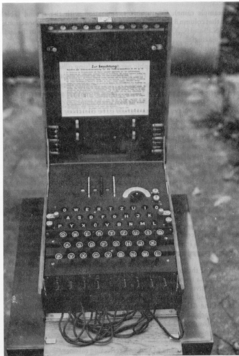
GERMAN ARMY MILITARY ENIGMA. THIS MODEL WAS THE MOST WIDELY USED VERSION OF THE GERMAN WAR-TIME ENIGMAS.
