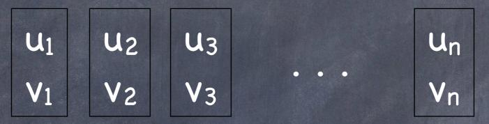
A solution is of this form: with the top and bottom strings identical.
